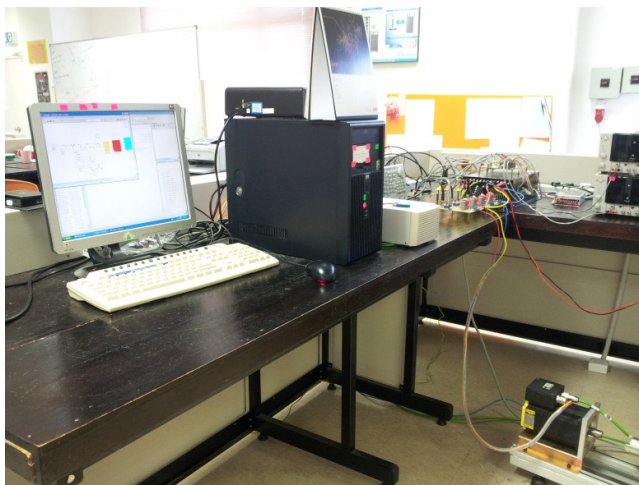
Fig. 3. Experimental set-up for sensorless speed control for PMSM drives
