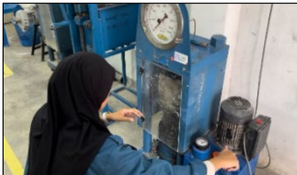
Rajah 1: Compression testing machine used to determine the compressive strength of the concrete specimen.
