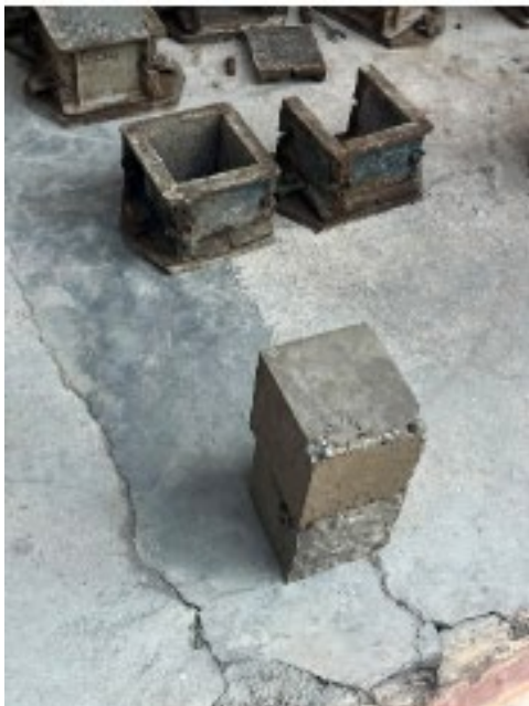
Rajah 1: Preparation of Concrete Samples Using LECA Balls
