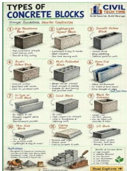
Rajah 1: Types of concrete block
