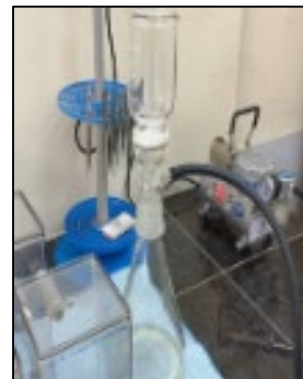
Rajah 2: Vacuum Filtration Apparatus for Total Suspended Solids (TSS) Analysis
