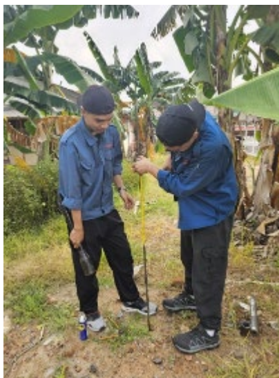
Rajah 1: Mackintosh Probe Test Work
