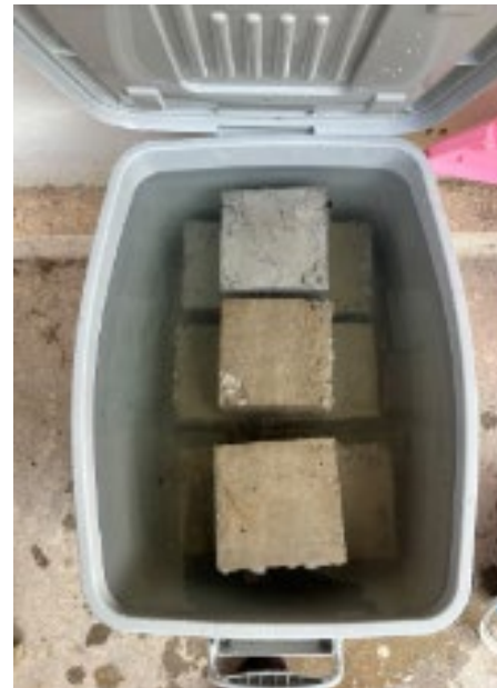
Rajah 2: Curing Process of Concrete Samples
