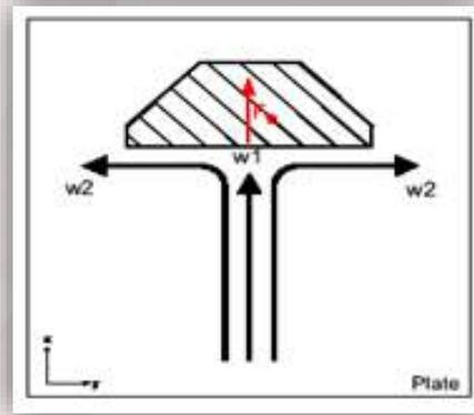
$$F_{th} = \rho Q x (v_1 - v_2)$$
