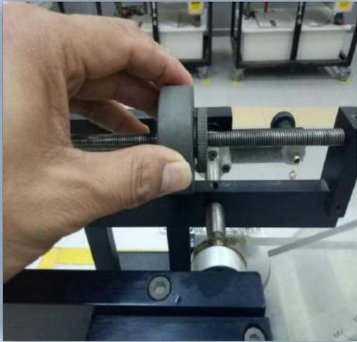
1. Set up the water vessel to an angle  $0^{\circ}$ . Counterbalance the unit with a rotating slider
