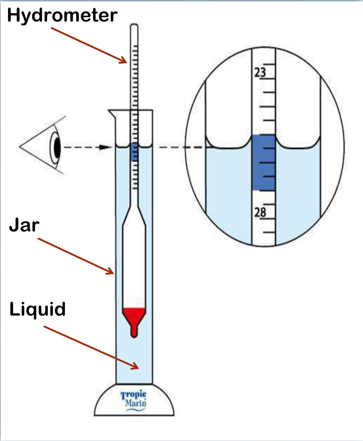
5. Accurate Reading Scale Method
