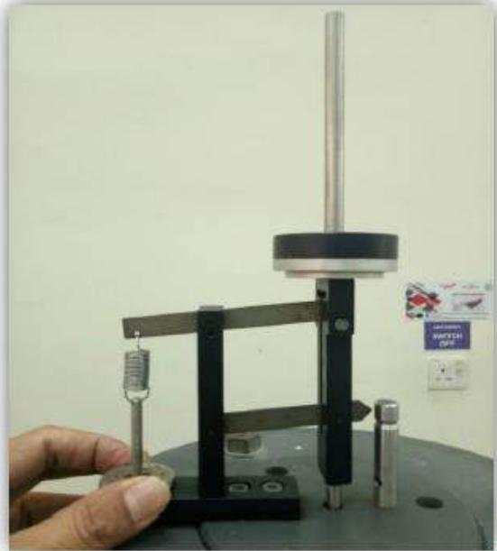
**2. Adjust Screw to pointer & Apply desired Loading**
