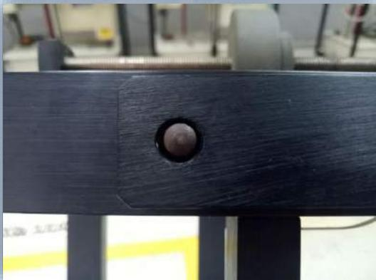
2. The stop pin precisely in the middle of the hole.
