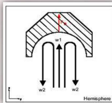
$$F_{th} = \rho Q x (v_1 - v_2)$$
