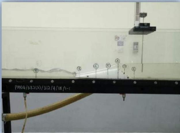
6. Measure the height of water from base of channel at every station
