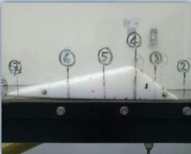
5. Measure the height of crump weir from base of channel at every station
