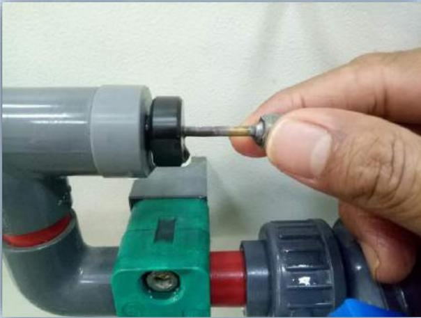
4. Move the probe to the centre of diameter for each measurement point
