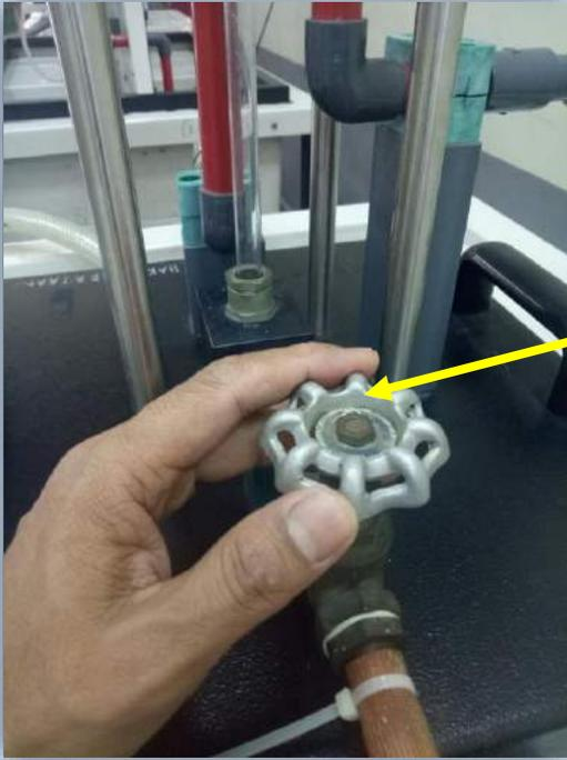
**4. Control Drain Valve for Laminar, Transition or Turbulent**
