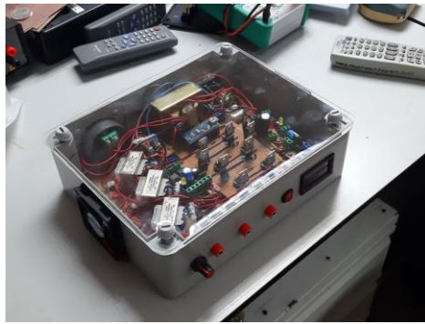
Figure 1 shows the corner view of Three Phase Motor Controller By Mosfet Using Arduino
