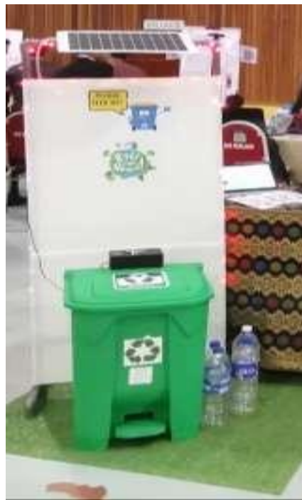
Figure 8: Prototype of The IOT Based Solar Powered Recycle Bin with Monitoring System
