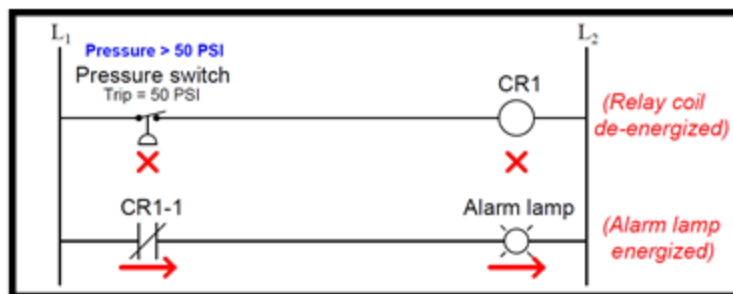
Figure 2.32: The pressure switch more than 50 PSI
