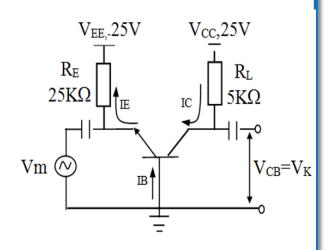
Determine the output voltage for common base amplifier above
