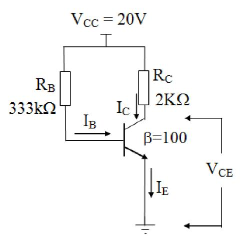
Figure : Common Emitter Amplifier Circuit
