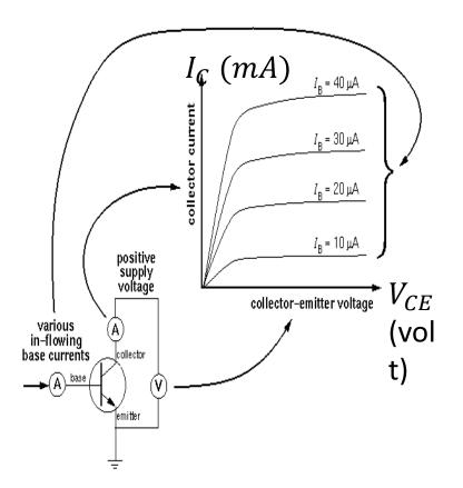
The I<sub>c</sub> - V<sub>c</sub> characteristic curve is the graph of a collector current versus collector voltage that describe the output of common emitter amplifier during any changes of voltage and current
