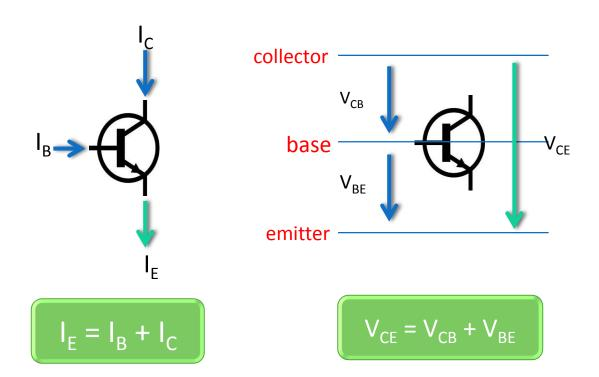
$V_{BE} = 0.7V \ (silicon)$  $V_{BE} = 0.3V \ (germanium)$  $V_{BE} = 0V \ (if not stated in question)$
