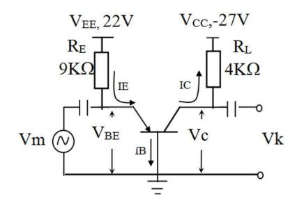
If silicon types of transistor are used. Determine the output voltage for common base amplifier above
