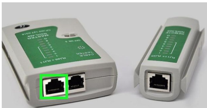
Figure A10: Plug both Ethernet cable end into cable tester
