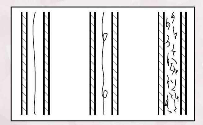
Figure 2: Three flow regimes: (a) laminar, (b) transitional & (c) turbulent
