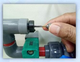
4. Move the probe to the centre of diameter for each measurement point
