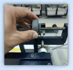
Set up the water vessel to an angle 0°. Counterbalance the unit with a rotating slider
