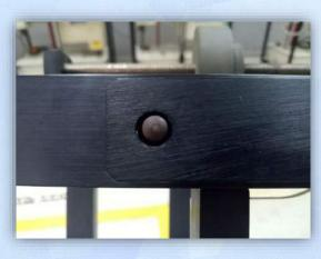
2. The stop pin precisely in the middle of the hole.
