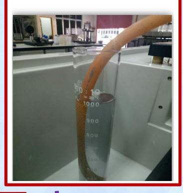
3. Stop Watch for record time (second) for water rise in measuring cylinder. Minimum is 1 liter
