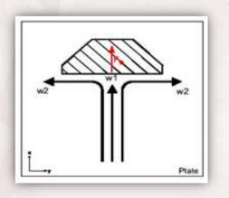
Fth =  $\rho Q x (v_1 - v_2)$ if  $v_2 = 0$  then Fth =  $\rho Q \cdot v_1$
