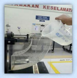
5. Pour water to the vessel until the unit is balance (stop pin at the middle)
