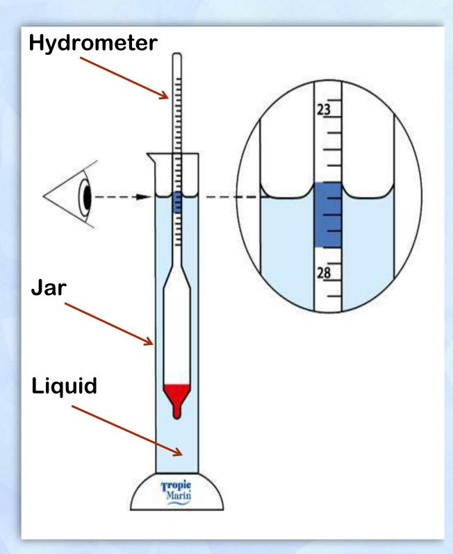
5. Accurate Reading Scale Method
