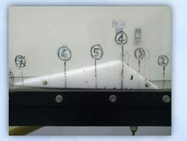
5. Measure the height of crump weir from base of channel at every station
