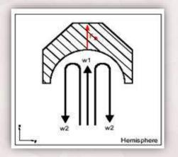
Fth =  $\rho$  Q x (v<sub>1</sub> - v<sub>2</sub>) if v<sub>2</sub> = - v<sub>1</sub> then Fth =  $\rho$  Q . 2v<sub>1</sub> PW5
