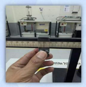
3. Place the Hanger to the Lever Arm and set Lever arm on the Scale
