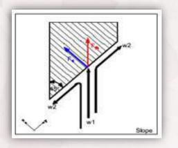
$Fx = \rho Q x (v_1 \cos \alpha)$  $Fth = F_x \cos \alpha$  $with \alpha = 45^0$  $Fth = \rho Q \cdot v_1 \cdot \cos^2 \alpha$
