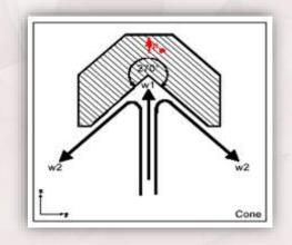
Fth =  $\rho Q x (v_1 - v_{2x})$ if  $v_2 = -v_1 \cos \alpha$  with  $\alpha = 45^{\circ}$  $v_{2x} = v_2 \cos \alpha$ Fth =  $\rho Q \cdot v_1 (1 + \cos^2 \alpha)$
