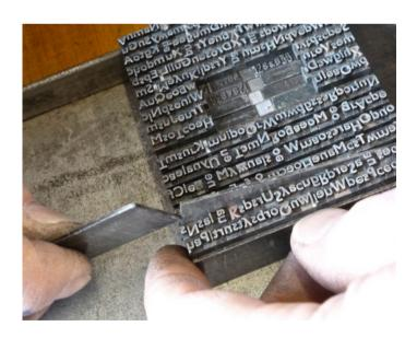
Figure 8: Lead sheets used to space font arrangement (Source: sifoo.com)
